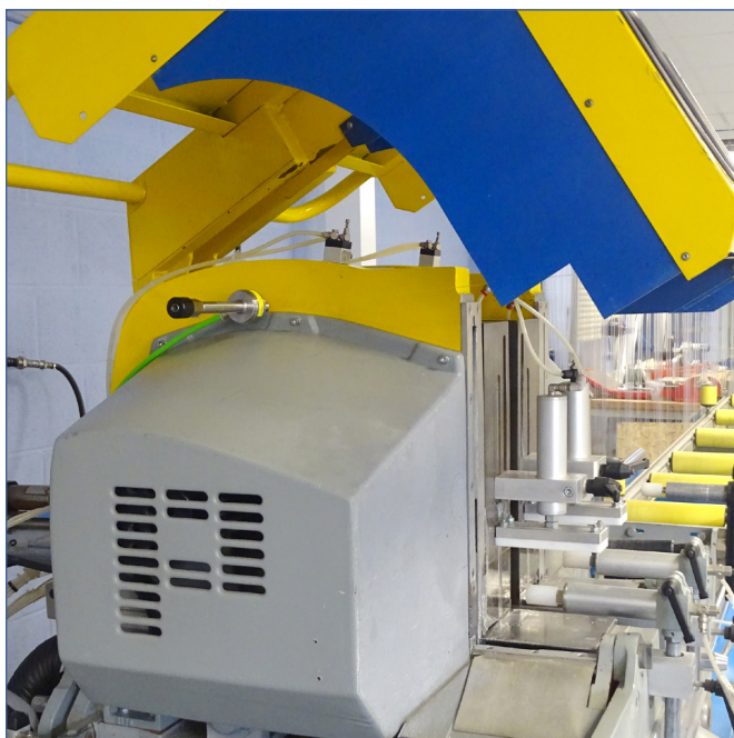
Vortex Tube used to cool saw blade.
