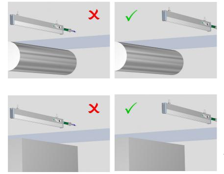
2. Avoid proximity to earthed parts of machinery as this will distort the corona and reduce its efficiency.
