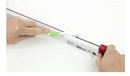
lonising bars will need periodic wiping to clean grey deposits from the surface of the bar. A cloth moistened with a small amount of IPA or methylated spirits is recommended. Allow a moment to dry before switching on.
