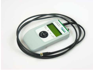
BarMaster remote programmer. Allows optimisation of the output of the 924EX
