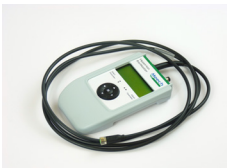
BarMaster remote programmer. Allows optimisation of the output of the 971IPS-30
