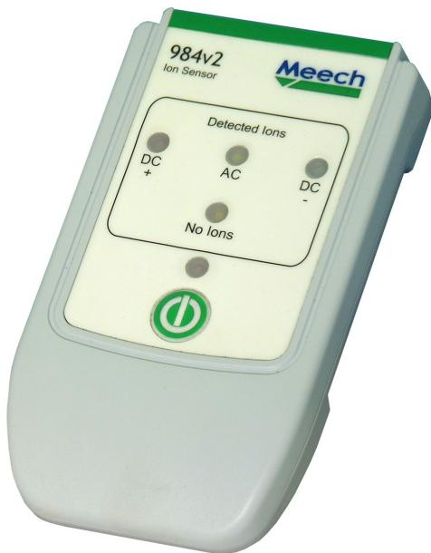
The Meech Model 984v2 has been developed for inspection and maintenance engineers. It is an easy to use tool to verify the operation of both AC and DC powered static elimination bars. The Model 984v2 features a series of indicator lights to show whether ions are being emitted from a static eliminator bar.
