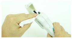
The emitter pins must be allowed to dry before the cap is replaced. Before reactivating the Ion Gun ensure that the nozzle cap is correctly latched by locating the retaining clip over its lug and pressing down lightly.
