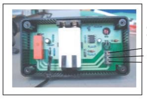
Output relay connections
