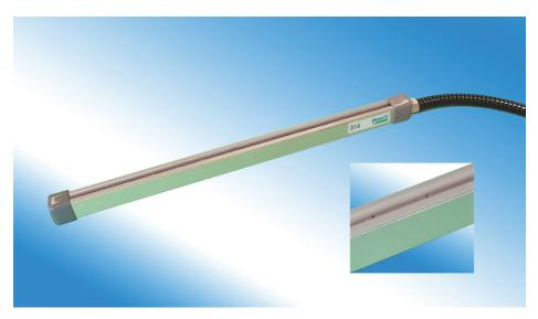
The Meech Model 914EX has been designed to meet the most arduous of static elimination problems. The special resistive coupling of its emitter pins renders them shockless, whilst giving powerful static neutralisation performance. This enables the Bar to eliminate very high static charges on high speed webs and at longer ranges than has been previously possible.
