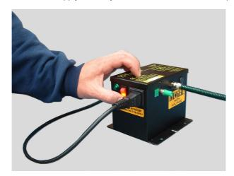
1. Switch off the electrical supply to the system and disconnect the IEC plug.
