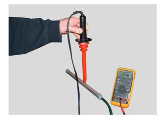
6. If the voltage is below 4.0 kV then the bar should be returned to Meech for service and/or repair.
