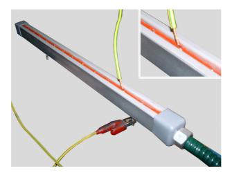
As the spark is drawn a slight buzzing sound will also be heard. This indicates that the bar is functioning correctly.
