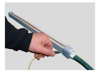
Holding the wire insulation, approach any of the bar emitter pins with the bare end of the wire.
