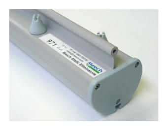
The profile of the 971 bar is rounded, with minimal dirt traps, making it useful for cleanroom applications. The bar has good rigidity, allowing it to span wide widths. Mounting is by M4x20 T bolts in a slot at the rear of the bar.
