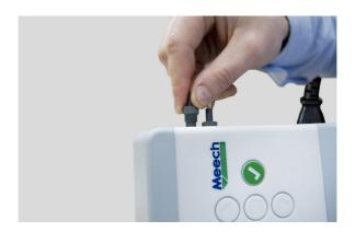
6. Using a high voltage probe (RS 610 281) and meter (RS 610 590) measure the voltage on the pins of the bar. This voltage should be between 3 and 6kV.
