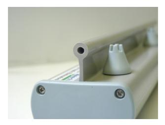
The upstand between the nozzles is a vital feature of the 971 bar. By increasing the tracking distance between positive and negative pins, the upstand helps maintain good performance even when the bar is contaminated.
