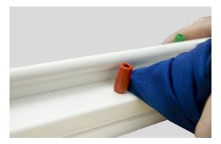
Let dry for a minute and replace the outer cap. Re-assemble the emitter pin onto the bar and turn back on.
