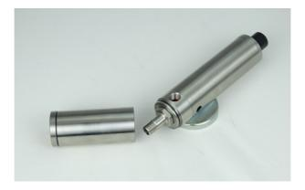
You will then need to remove the cold cap from the Vortex Tube. You can simply unscrew this from the ColdStream Gun. Inside you will find an O'ring and Generator.
