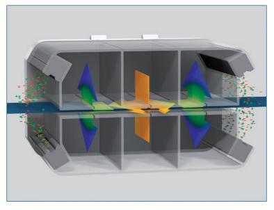
As the web exits the CyClean head, it passes through a second cloud of ionisation to prevent re-contamination of the web.
