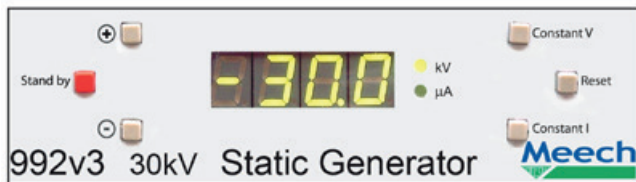
Display with 992v3 operating in Constant Voltage Mode
