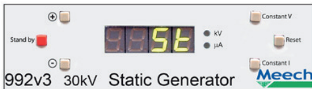
Display with 992v3 in Stand by function
