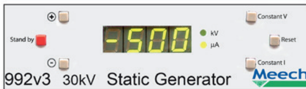
Display with 992v3 operating in Constant Current Mode
