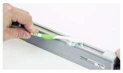
lonising bars will need periodic wiping to clean grey deposits from the surface of the bar. A cloth moistened with a small amount of IPA or methylated spirits is recommended. Allow a moment to dry before switching back on.
