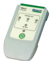
The 984v2 Ion Sensor is a device used for checking the performance of both AC and DC powered static elimination bars. Indicator lights confirm the presence of ions, and in the case of a DC power source their polarity. Regular monitoring of installations with the 984v2 will indicate when bars require cleaning or other maintenance work.
