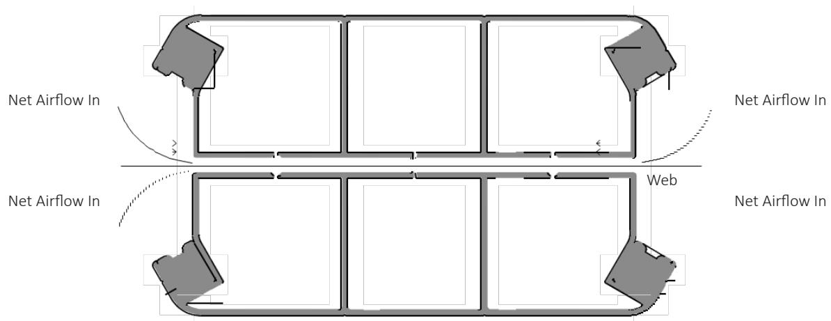
The net airflow into either side of the CyClean head is adjusted by bleeding off a volume of the blowing (positive) airflow to create an airflow bias in favour of vacuum.
