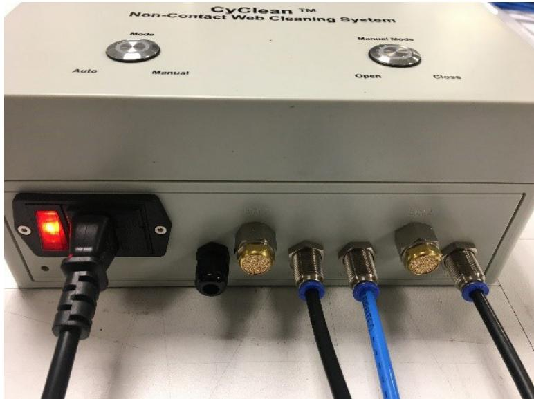
The compressed air hoses (blue and black) should be connected from the CyClean unit to the 6mm compressed air push fittings labelled Port 2 and Port 3. The blue hose connects to port 2, the black hose connects to Port 3.
