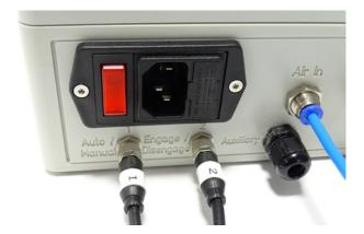
Connect plug 1 from the TakClean to the Auto/Manual socket on the pneumatic control box.
