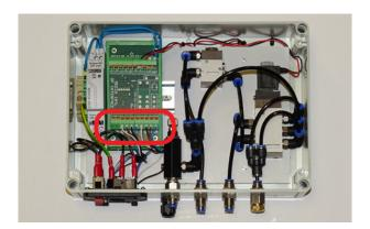
This can be fed into the pneumatic control box via the Auxiliary cable gland.
