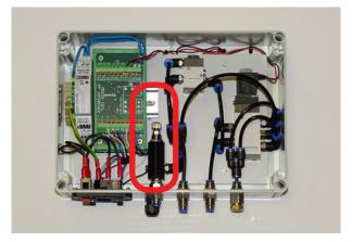
This valve will have been set at Meech before your system was supplied, so that the bottom adhesive roll engages the bottom TransTak elastomer roller with the required level of force.
