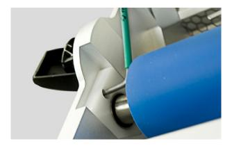
To remove the top TransTak roller, loosen the fixing screw located under the bearing carriers at either end of the TransTak roller. Support the TransTak roller whilst completing this operation so that it does not fall from its position. A 2.5mm Allen key is required to loosen the fixing screws.
