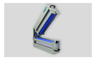
To remove the bottom TransTak roller, loosen the fixing screw located in the bearing carriers at either end of the TransTak roller. A 2.5mm Allen key is required to loosen the fixing screws.
