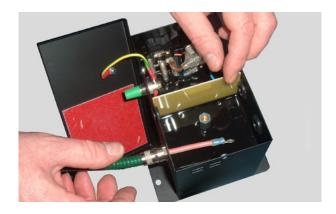
Then refit both the lock washer and nut to the ionising bar. Ensure that the nut is fully tightened.
