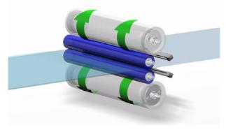
3. Any static charge present on the web is neutralised on exit from the TakClean; minimising the risk of statically attracted recontamination.
