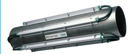
The 913 Flow Tube neutralises static charges on materials in handling and conveying systems. It incorporates in-line ionisation, which eliminates material clinging and clogging in ducting systems due to static charges. The 913 Flow Tube is powered by 905 power supply and is provided in a range of diameters to fit most of the industrial standard installations.
