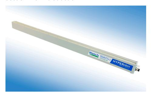
The Hyperion 924IPSv2 is a compact pulsed DC ionising bar. It is used to control static electric charges in short range applications (20-150mm). An integral 7.5kV pulsed DC power supply allows for easy installation on printing, converting and packaging machinery. Requiring only a 24V DC supply, the 924IPSv2 removes the need to route high-voltage cabling through the machine.
