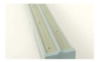
The 924IPSv2 is designed to operate in dirty, factory environments. To maximise the interval between cleaning the bar features a divider to increase the surface tracking distance between the two rows of high voltage pins. It is important to clean this area during cleaning operations.
