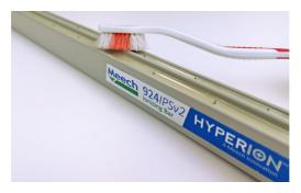
Ionising bars will need periodic wiping to clean grey deposits from the surface of the bar. A cloth moistened with a small amount of IPA or methylated spirits is recommended. Let dry for a minute and turn back on.
