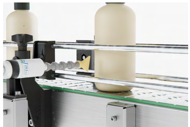
Image1: Dust contamination on print surface with surface cleaning application
